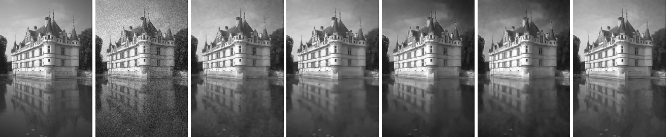
Figure 2. Image denoising example. From left to right: original image, image corrupted with additive Gaussian noise with \sigma = 25 , PSNR=20.17; our result, PSNR=28.94, 0.6 seconds and Fields of Experts result [18], PSNR=28.67, 2280 seconds; wavelet denoising [16], PSNR=29.05, 16 seconds; overcomplete DCT, PSNR=28.81, 38 seconds, and BM3D [6], PSNR=29.60, 4.3 seconds.
